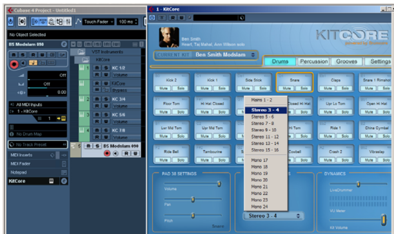
Figure 8. Assigning the Snare pad output to Stereo 3-4 to play through the corresponding audio track in Cubase
