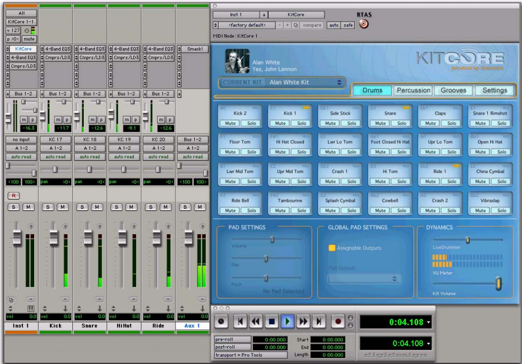
Figure 1. Example of a Pro Tools session with different KitCore Pads assigned to different outputs
